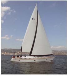
Double spreader Selden mast, choice of conventional, furling or fully battened mainsail, adjustable pneumatic boom vang and top quality deck hardware
