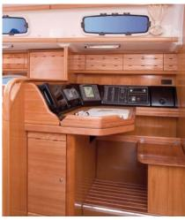
• Chart table with large compartment for charts and wrap around console for navigational instruments
